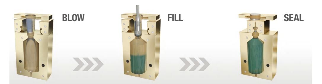
In the sterile filling area the parison is formed to final shape by blowing sterile compressed air into the parison. This process is supported by applying vacuum from the mold. The sterile product is filled in the container by the combined blowing/venting/filling nozzles.
