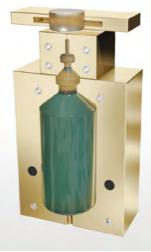
In the final step the container is hermetically sealed by the sealing molds and discharged from the machine.
