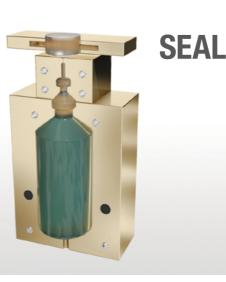
In the final step the container is hermetically sealed by the sealing molds and discharged from the machine.
